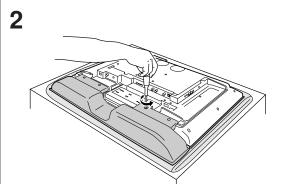
Unfasten the four screws used to secure the speaker in place.
